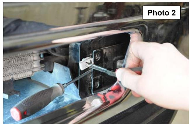
3. Place bracket behind frame horn. (with the light tab to the inside). **See Photos 3 & 4.**
